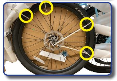
Carefully remove the front tire from the bike by sliding it directly forward, to avoid damaging the spokes or pedal arm. Then remove the front fender from the tire and set both aside.
