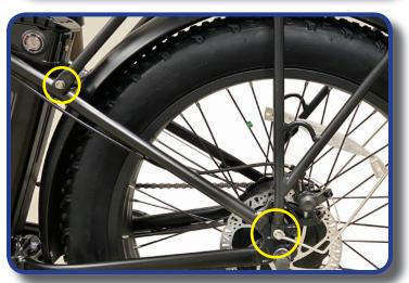
Feed the rear tail light wire through the rear rack as shown. Once the wire is in place, plug it into the tail light by lining up the two arrows on the connectors.
