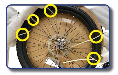
Carefully remove the front tire from the bike by sliding it directly forward, to avoid damaging the spokes or pedal arm. Then remove the front fender from the tire and set both aside.
