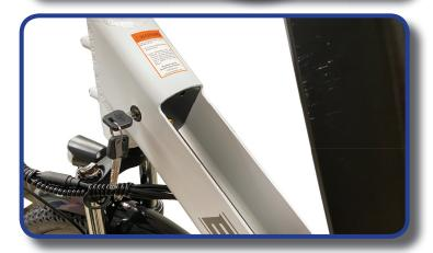
With the battery removed, check your battery's state of charge by pressing the red button.
